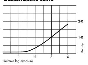
100 DELTA Professional rollfilm developed in ILFORD ID-11 stock for 8½ minutes at 20°C/68°F with intermittent agitation. This curve is also representative of the 35mm and sheet film formats.
