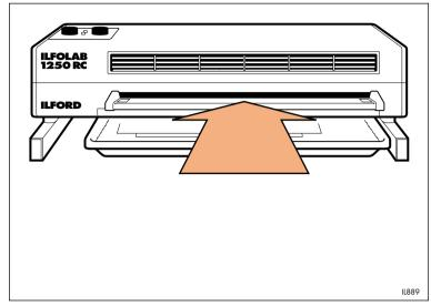
**3** Feed prints emulsion side up. Ensure prints are fed squarely. Feed small prints with the short edge leading. Do not overlap one print with another - allow 2 seconds between the trailing edge of one print and the leading edge of the next.
