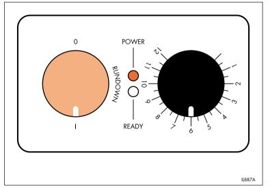
**1** Switch the electrical supply on. Turn the dryer control to 'I'. The red 'POWER' light illuminates.
