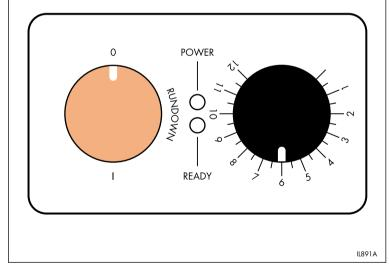
**2** To switch the dryer off completely, carry out operation 1 and wait for the fans and main drive to stop. Then turn the dryer control to 'O'. Switch the electrical supply off.
