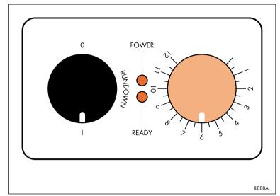
**2** Allow about  $1\frac{1}{2}$  minutes for the orange 'READY' light to switch on. As a guide, set the speed control to position 6 to dry resin coated paper sheets.
