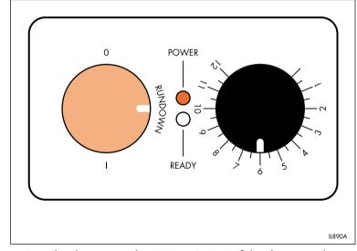
■ Turn the dryer control to 'RUNDOWN'. If the dryer is to be used again later the same day, the control can be left in this position.
