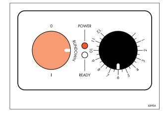
2 To switch the dryer off completely, select 'RUNDOWN' and wait for the fans and main drive to stop. Then turn the dryer control to 'O'. Switch the electrical supply off.
