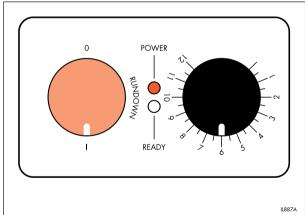
2 Allow about  $1^{1}/_{2}$  minutes for the orange 'READY' light to switch on. During this time, transfer the washed prints to the wet-print dish. As a guide, set the speed control to position 6 to dry resin coated paper sheets.
