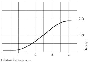
FP4 Plus rollfilm developed in ILFORD ILFOTEC HC (1+31) for 8 minutes at 20°C/68°F with intermittent agitation. This curve is also representative of the 35mm and sheet film formats.
