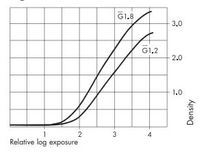
ORTHO Plus copy film developed in ILFORD PHENISOL (1+4) for 3 minutes and 10 minutes, at 20°C/68°F with intermittent agitation.
