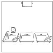
Set up your safelight (e.g. the ILFORD SL1 safelight) at least 1.2m/4ft from the developing dish. Lay out three processing dishes, label them DEV, STOP and FIX, two pairs of print tongs, and a clock for timing development. Then mix up the processing chemicals using water at about 23°C/73°F. The aim is to process at a working temperature of 20°C/68°F +/- 1°C/2°F, so a few degrees are allowed for heat lost in mixing and cooling.
