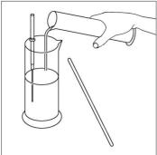
Mix up the developer solution 1+9 by measuring out 60ml of ILFORD MULTIGRADE developer in a 150ml cylinder, and adding this to 540ml of water in a 600ml cylinder. For the stop bath, add 30ml of ILFORD ILFOSTOP stop bath to 570ml of water (1+19). For fixing, add 120ml of ILFORD RAPID FIXER to 480ml of water (1+4). (This gives enough processing solutions to process about 40 20.3x25.4cm/8x10in MULTIGRADE RC prints).
