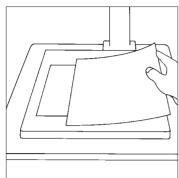
With the safelight on, and the room lights off, put a sheet of MULTIGRADE paper into the easel, shiny side up. (Reseal the packet carefully.) You are now ready to make a test print. Switch on the enlarger lamp and expose the whole sheet for two seconds. Cover one-quarter of the sheet with opaque card, and expose the rest for another 2 seconds. Cover half of it, and expose the rest for another 4 seconds. Cover three-quarters, and expose the last part for another 8 seconds.
