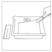
Repeat the processing steps (8-10) exactly as you did before. Again, check the temperature of the developer and time the development stage. If the developer has cooled more than a few degrees, warm it up by pouring it into a 600ml cylinder and running hot water over the outside of it. (The temperature of the stop and fix are not as critical.)
