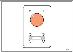
1 At the end of the working period, turn the processor control switch to 'O'.
