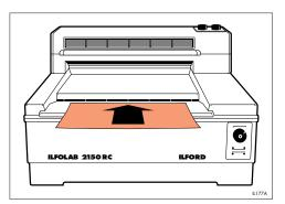
3 When 'ready' light is steady on, feed sheets emulsion side down with long edge leading. Wait for the audible signal before feeding in the next sheet.
