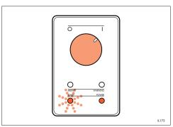
1 Ensure processor lid is closed, water and electrical supplies are on. Turn processor control switch to '|'.
