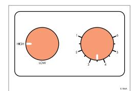
2 Adjust dryer temperature to establish the optimum setting. Select High for gloss papers, select low for matt or pearl papers. Start at position 3.5 and work from there.
