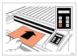
4 When the display reads STANDBY OFF and the LED is steady on, the processor is readv , ready for use. Feed sheets emulsion side down.
