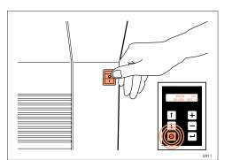
2 Switch the processor on. The display reads W A R M and the ready LED flashes, UΡ indicating the processor is not
