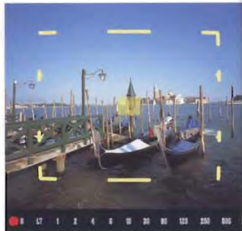
Viewfinder Display for 80mm Lens. Bright field of view frame with panoramic markings. Bright RF area in center. Bottom shows red warning light on left, shutter speeds in center and over-exposure signal on right.
