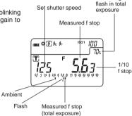
5. When the light from the flash is received, the measured value (f stop) is displayed. Even after measurement, the mode mark ② continues to blink and the meter is in ready state and a new measurement can be made. (Auto-reset function)
