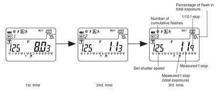
To clear the cumulative value, press M. CLEAR button (2) or switch to another mode by turning the Jog wheel while pressing the Mode button.
