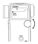
Press the Measuring button to trigger the flash. The measured value (f stop value) will be displayed.
