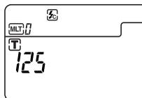
4. Press the Measuring button
